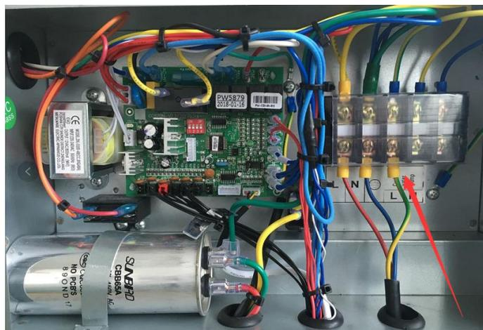
**Note:** In the case of three-phase models, swapping two phases may cause the electric motors to run in the reverse direction, which can lead to damage. For this reason, the unit has a built-in protective device that breaks the circuit if the connection is not correct. If the red LED above this safety device lights up, **you must swap the connections of two of the phase wires.**
