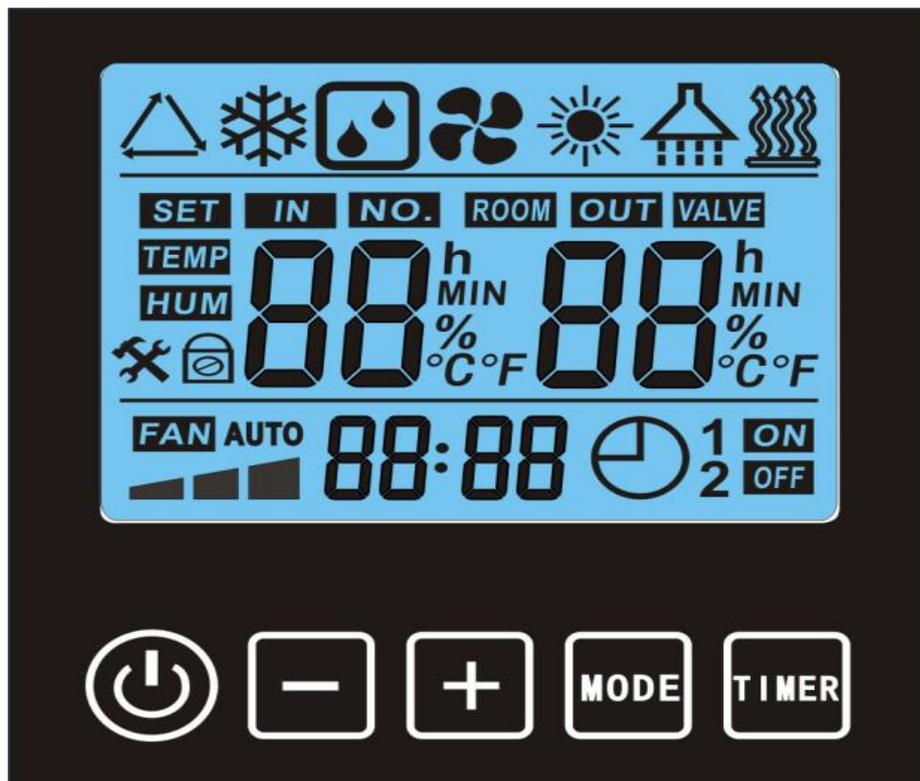
When the heat pump is running or standby, the LED display shows the inlet water temperature and setting temperature.
